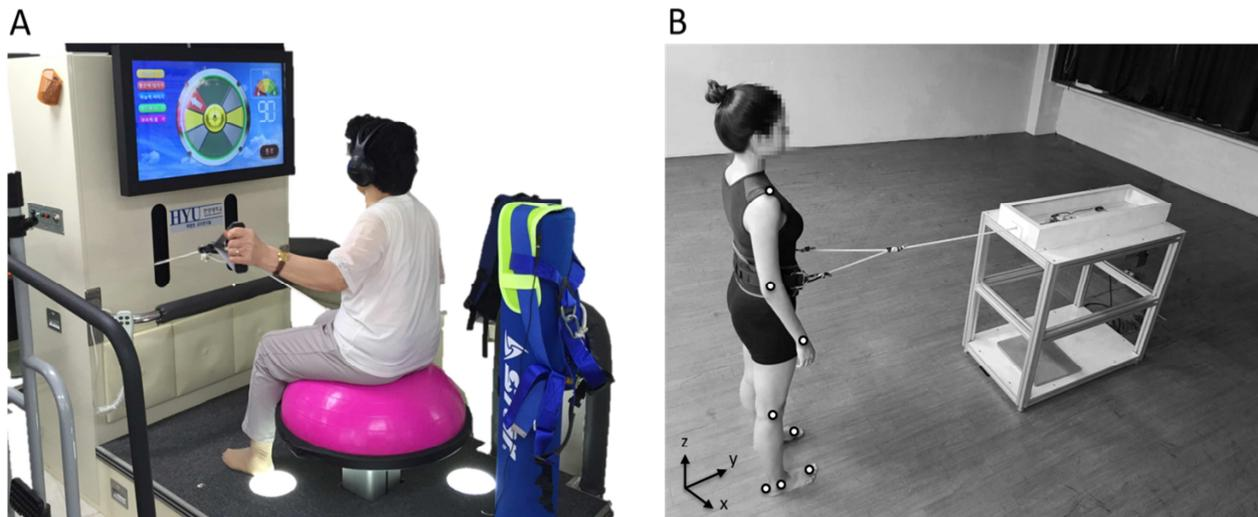
**Figure 1.** (A) shows a core exercise training equipment for elderly. (B) shows an experiment setup using a perturbation device.
